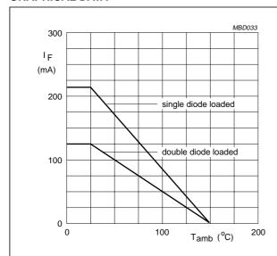
Device mounted on an FR4 printed-circuit board.
